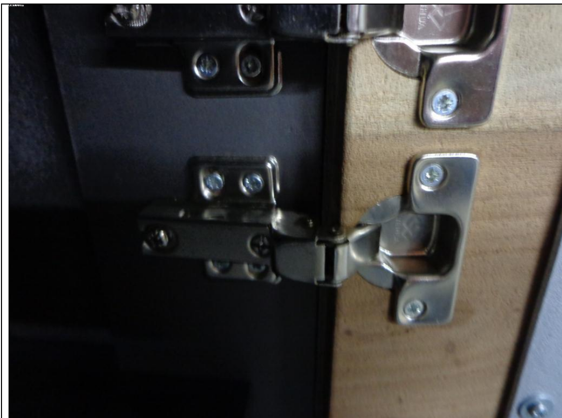
Adjustable , soft closing hinges.
